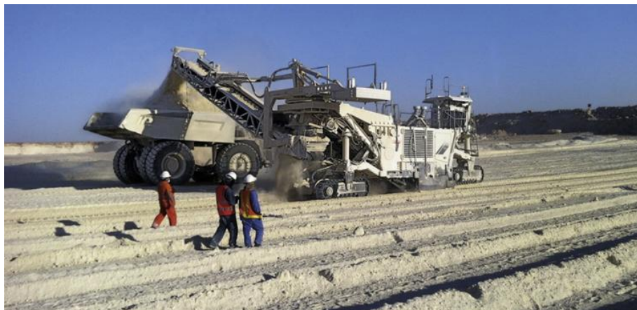
Fig 1 - Example Surface Miner – Limestone row cutting
