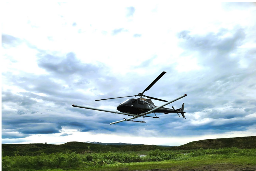
Figure 1. Airborne Geophysics surveying at 50 metre line spacing across the Caribou Dome during July 2025
