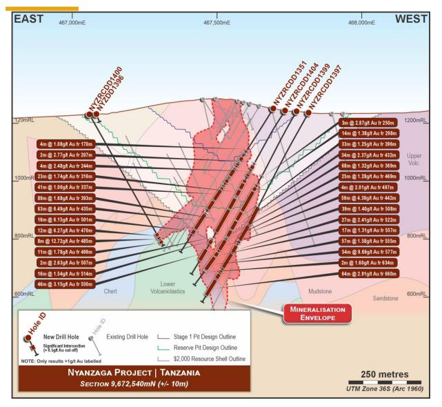
Figure 7: Tusker Deposit - cross section at 9,672,540mN looking north showing selected new intercepts and historical drill traces on simplified geology
