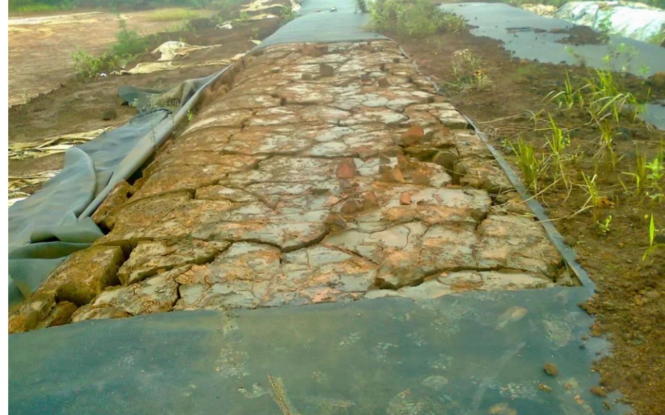
An example of acidic \text{TiO}_2 waste sludge after dewatering
