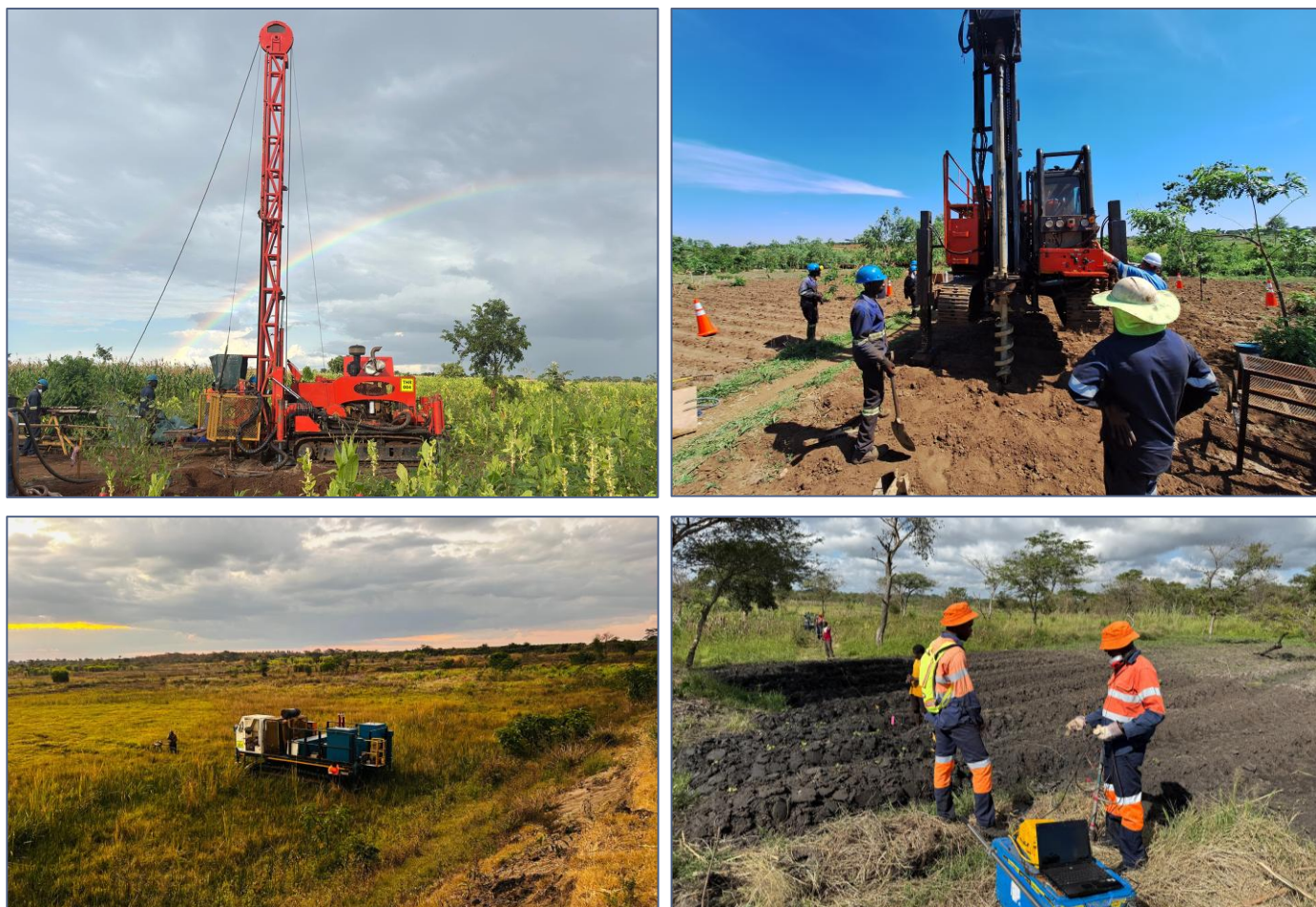
Figures 1-4 Clockwise from Top Left: Geotechnical diamond drilling, auger drilling, seismic geophysics testing using multi-channel analysis of surface waves (MASW), Cone Penetration Test with pore pressure measurements (CPTu) rig.
