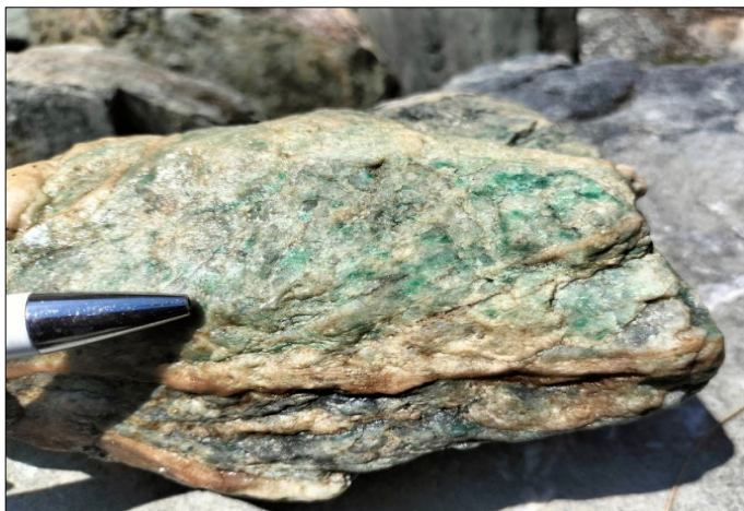
Image 5* (left) – Siliceous green schist with malachite staining and chalcopyrite-pyrite inclusions.
