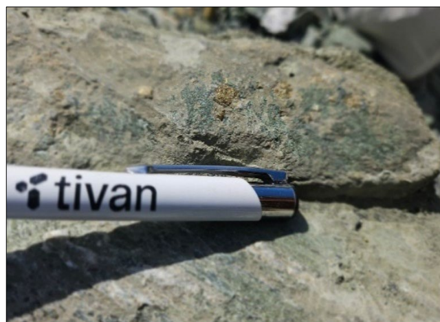
Image 3* (left) – Green schist foliation-hosted chalcopyrite and coarse pyrite within quartz veining. Image 4* (right) – Foliated black schist with groundmass hosted chalcopyrite and pyrite inclusions.
