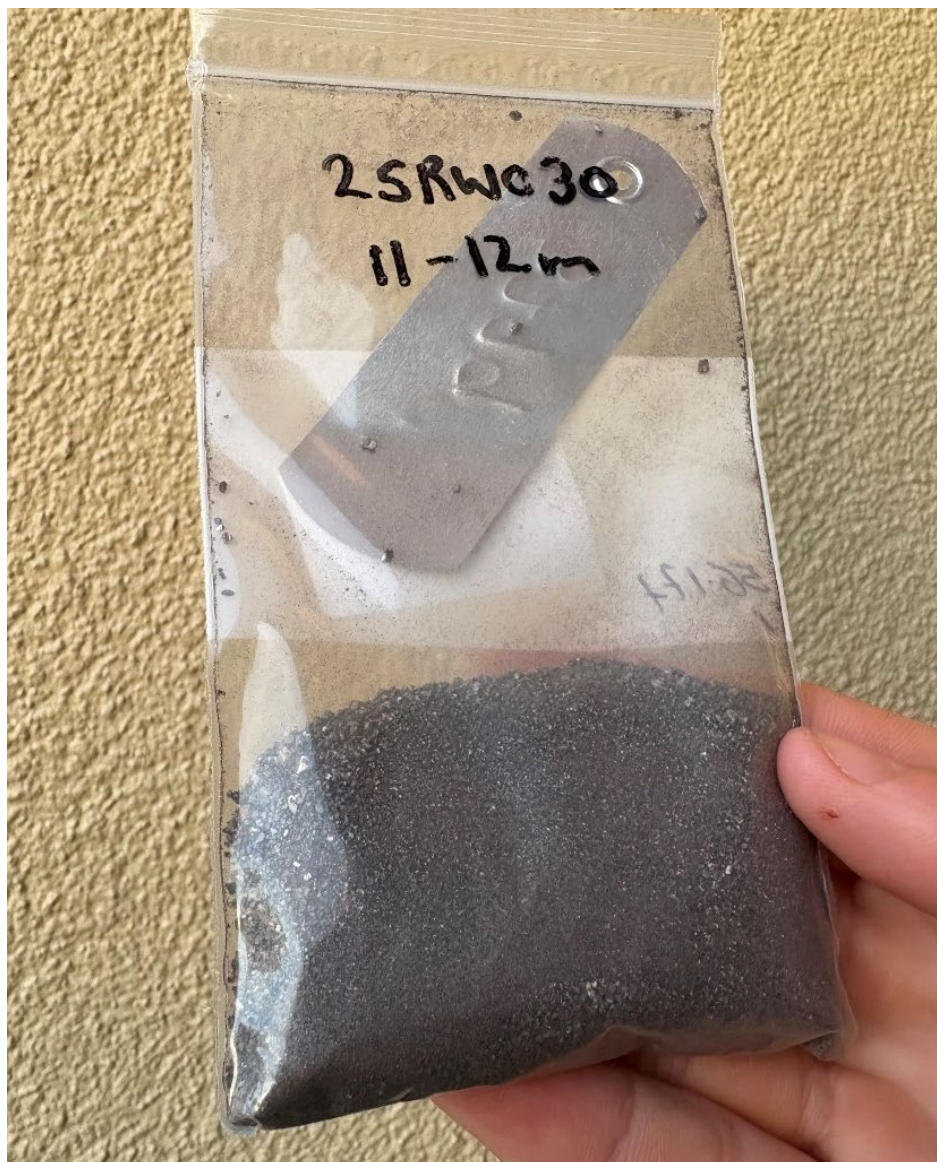
Photo 1 – Exceptional HMC sample from Drill hole 25RW030 returning 55.7% HM from 11-12m.
