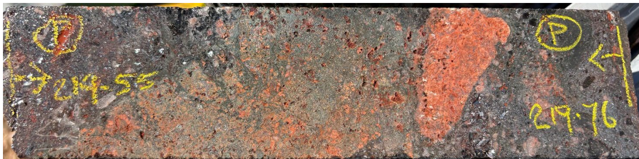
Figure 15. HMBDD003, ~219.6m. Vein breccia in altered granite with earthy hematite after an unknown mineral in clasts. Down-hole is to the right.
