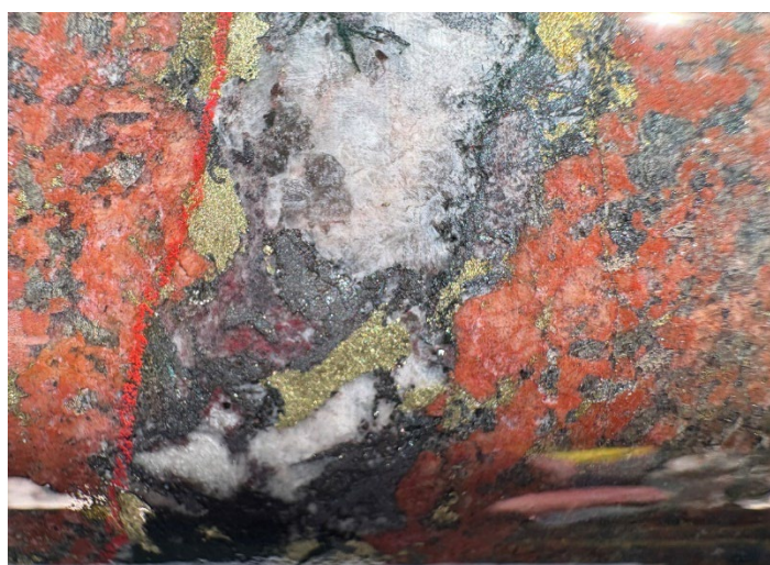
Figure 16. HMBDD003, ~474m. Calcite, magnetite, hematite vein with pyrite and chalcopyrite.
