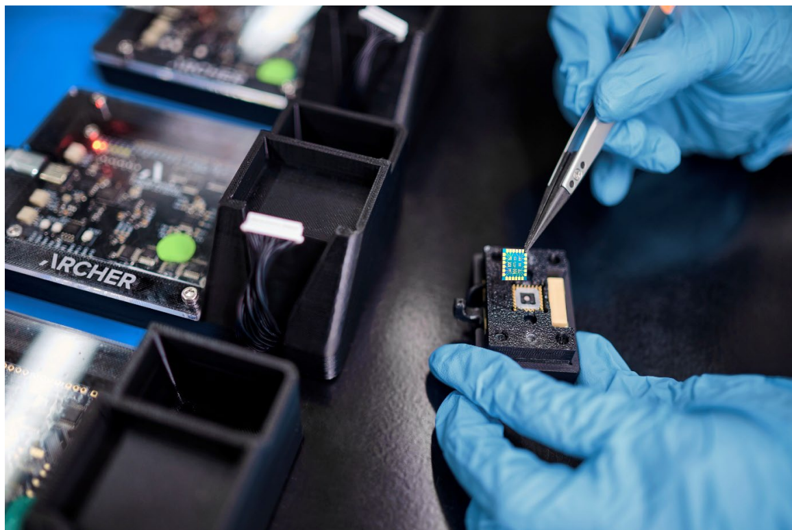
Image 1: Archer's lab biochip testing systems in Sydney. An engineer is placing prototype biochips into our fluidic system which then gets connected to the electronic readout system. The bolstered engineering team along with increased testing capability, like the setups above, is accelerating the development.
