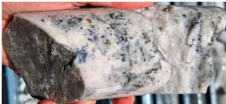
SDDSC161 intercept: 0.2 m @ 4,700 g/t Au and 0.26% Sb from 511.3 m showing abundant visible gold in a quartz-carbonate-stibnite vein. Part of a wider zone grading 3.4 m @ 466.4 g/t AuEq (466.0 g/t Au, 0.2% Sb) from 508.4 m. Core diameter is 63.5 mm.
