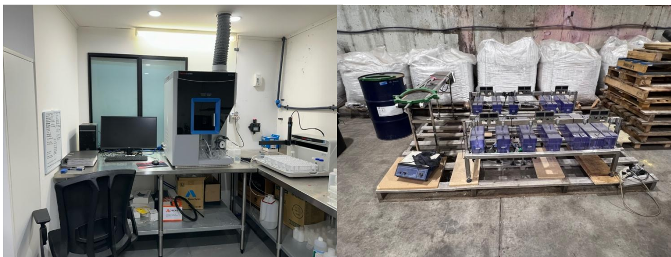
Figure 9 (L). ICP analytical machine capable of reading up to 66 elements to ppb levels of detection.
