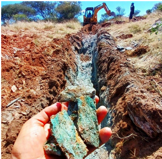
Photo 1 (left): Copper oxide mineralisation in schist – DET003 2-5m 5 Photo 2 (right): Copper oxides within ferruginous-calcite – DET003 61-62m 5
