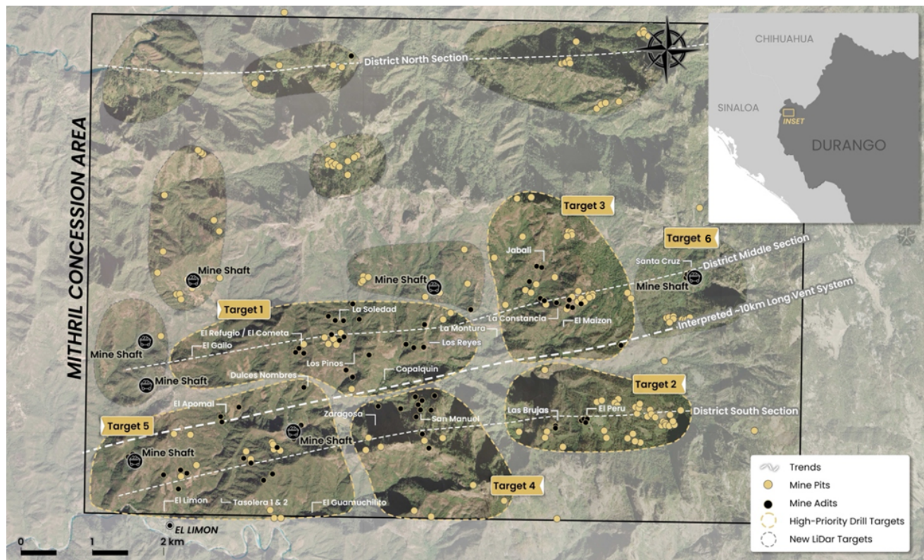
Figure 2 LiDAR identified historic workings across the 70km 2 district. Current drilling locations at Targets 1 and Zaragoza mine area, high priority drill target area of La Constancia-El Jabali (Target 3) and Target 5. Several new areas highlighted across the district for follow-up work including recently sampled Target 6
