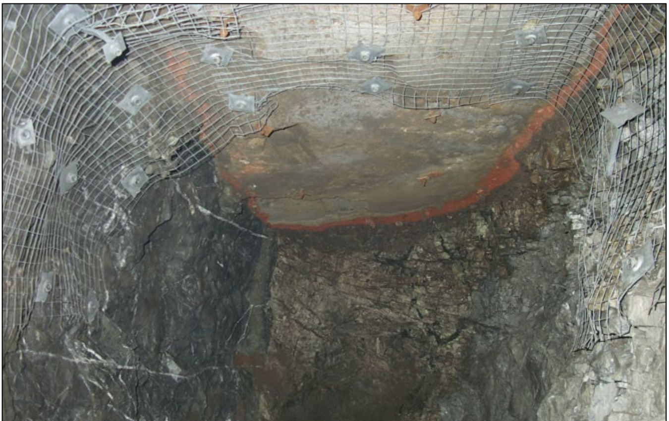
Figure 18: Example of Underhand Cut and Fill from the Black Swan nickel mine.
