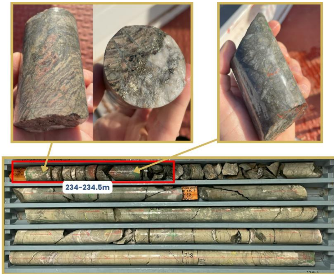
Figure 3: Diamond Tail of MGRC0018 from 234m. Mineralised BIF unit intercepted from 234 to 234.5m, with footwall alteration from 234.5 to 239m. See Appendix B - Table 3 for detailed descriptions and visual estimates. Assays Pending (estimated 4-6 weeks). Cautionary Statement: Visual estimates of mineral abundance should never be considered a proxy or substitute for laboratory analyses where concentrations or grades are the factor of principal economic interest. Visual estimates also potentially provide no information regarding impurities or deleterious physical properties relevant to valuations.
