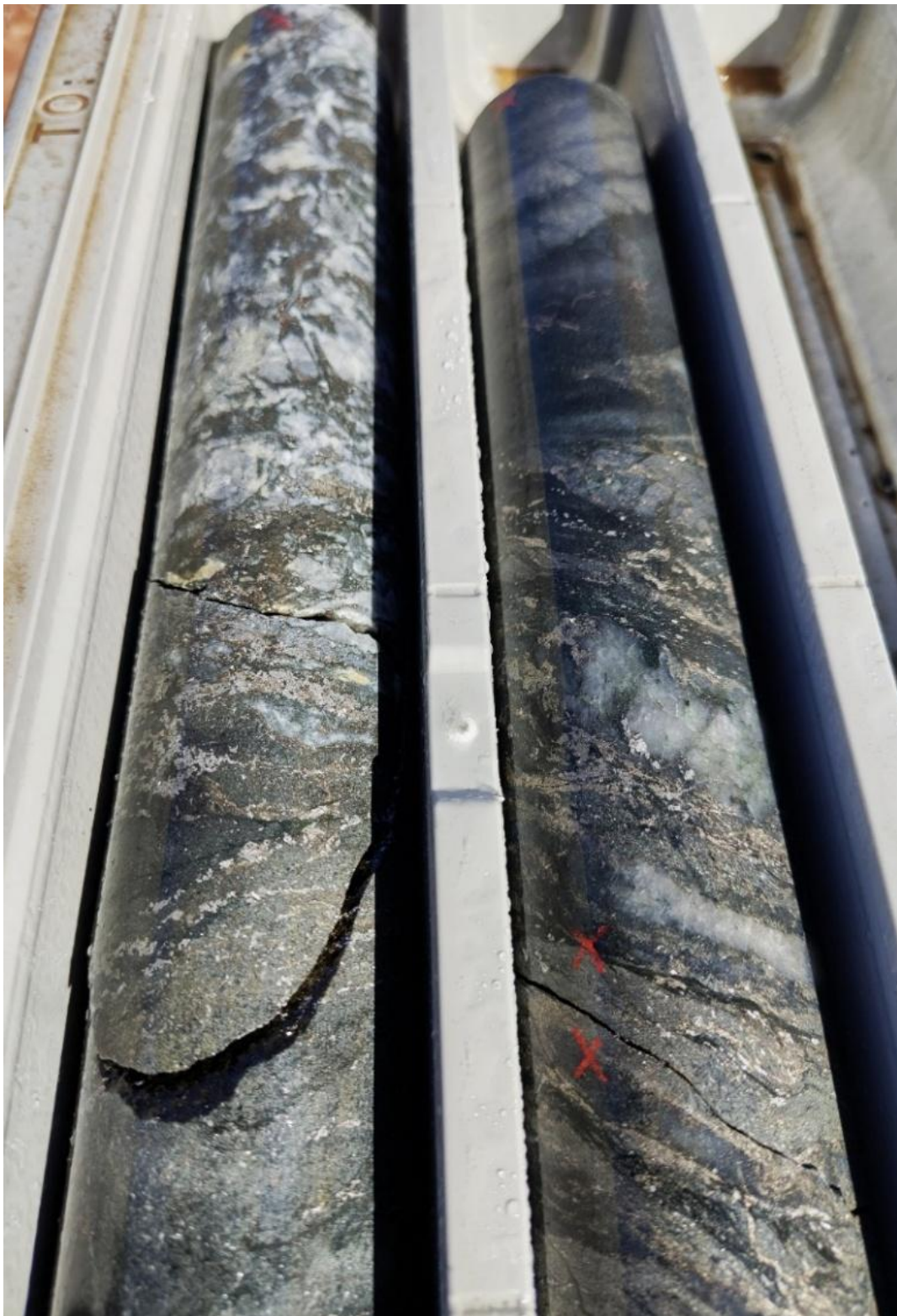
Photo 1. Typical higher-grade gold mineralisation at Main Hill from drill hole 25MYDD012. The NQ core (diameter 47.6mm for scale) is from 274-276m and is part of the intercept of 7m @ 2.66g/t Au. Left-hand core is 274-275m with grade of 4.12 g/t Au and the right-hand core is from 275-276m with grade of 2.9 g/t Au. Mineralisation within the BIF comprises quartz veining with associated pyrrhotite and arsenopyrite. Arsenopyrite is a key indicator of gold mineralisation. Note that extensive metallurgical test work indicates that mineralisation at Mt York is free-milling (see KAI press release dated 27 November 2024 entitled 'Strong Scoping Study forecasts robust financial returns').
