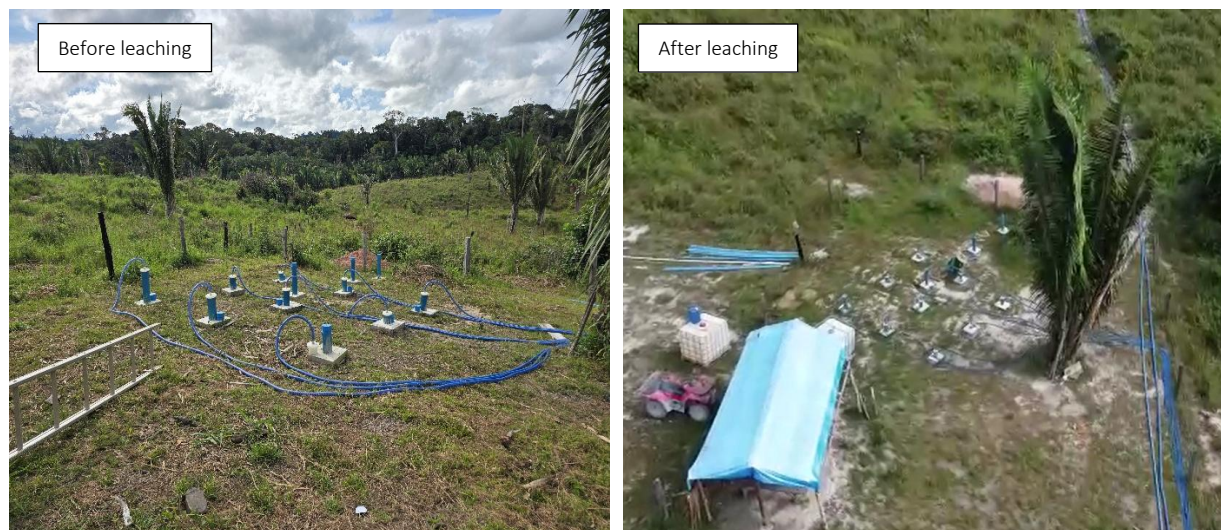
Figure 3. Before and after photos of the field pilot trial after 2 months of operation. Grass area was cut prior to leaching and vegetation and flora areas remain largely unaffected by the ISR process, other than by heavy foot traffic.
