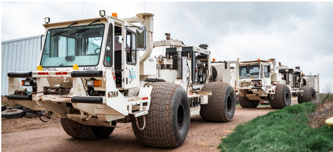
Figure 5. Paragon Geophysical Vibroseis trucks on location within survey area.
