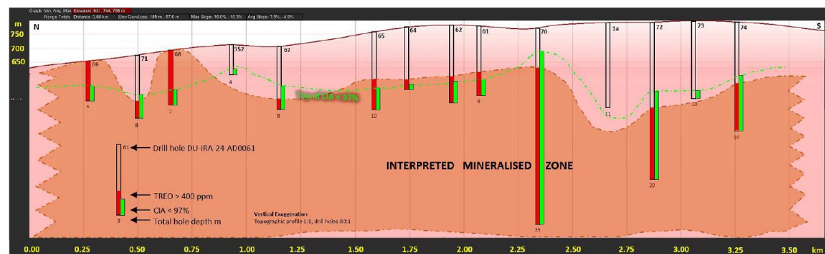
Figure 1. Drill hole section over 3 kilometres extent showing the intensity of weathering indicated by the Chemical index of Alteration in green (CIA, target zone is between 65% and 95%) together with zones of mineralisation in red above the cut off of 400 ppm TREO. Maximum values were up to 3362 ppm TREO with 69% Magnet REO/Total REO -CeO2.
