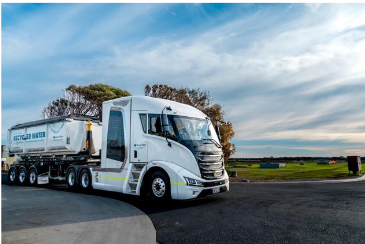
Image 2: The Taurus Hydrogen Fuel Cell Prime Mover with trailer attached
