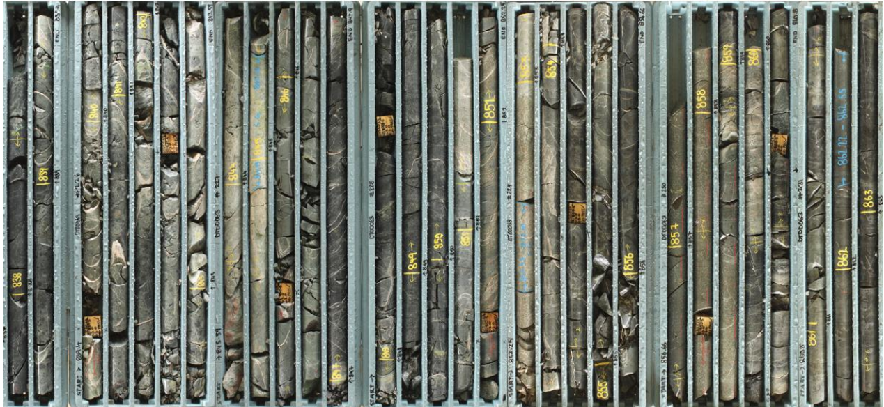
Figure 6 – Drill intersection of stockwork quartz and pyrite veins at 839 – 862m which is interpreted to be the down-plunge extension of the Duffer Lode.
