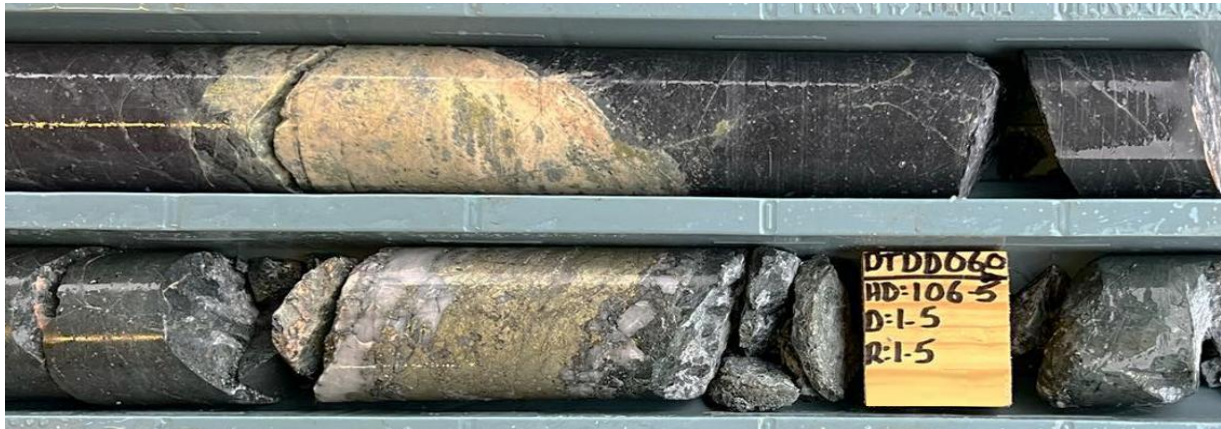
Figure 4 – Intersection of semi-massive chalcopyrite-pyrite-quartz vein in DTDD060 (106.15 – 106.65m).
