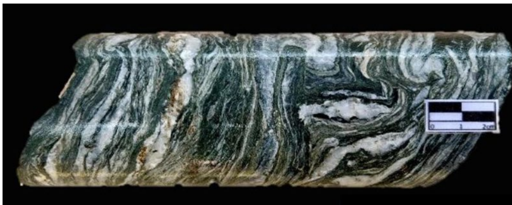
Figure 4: Hole BRD009 (at 112.4m): Photo shows example of intense ductile deformation manifest as mylonite, with shear foliation at 80° to CA. contains, boudinaged and locally tightly folded quartz veins (<1-1cm), pyrite and arsenopyrite are commonly present along the shear foliation planes. Note that the observed presence of such minerals or visual estimates of their abundance should never be considered a proxy or substitute for laboratory analyses where the concentrations or grades of gold mineralisation are the factor of principal economic interest. Visual estimates also potentially provide no information regarding impurities or deleterious physical properties relevant to valuation.
