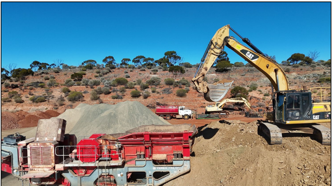
Figure 2: Ore being crushed at ROM - Menzies Gold Project
