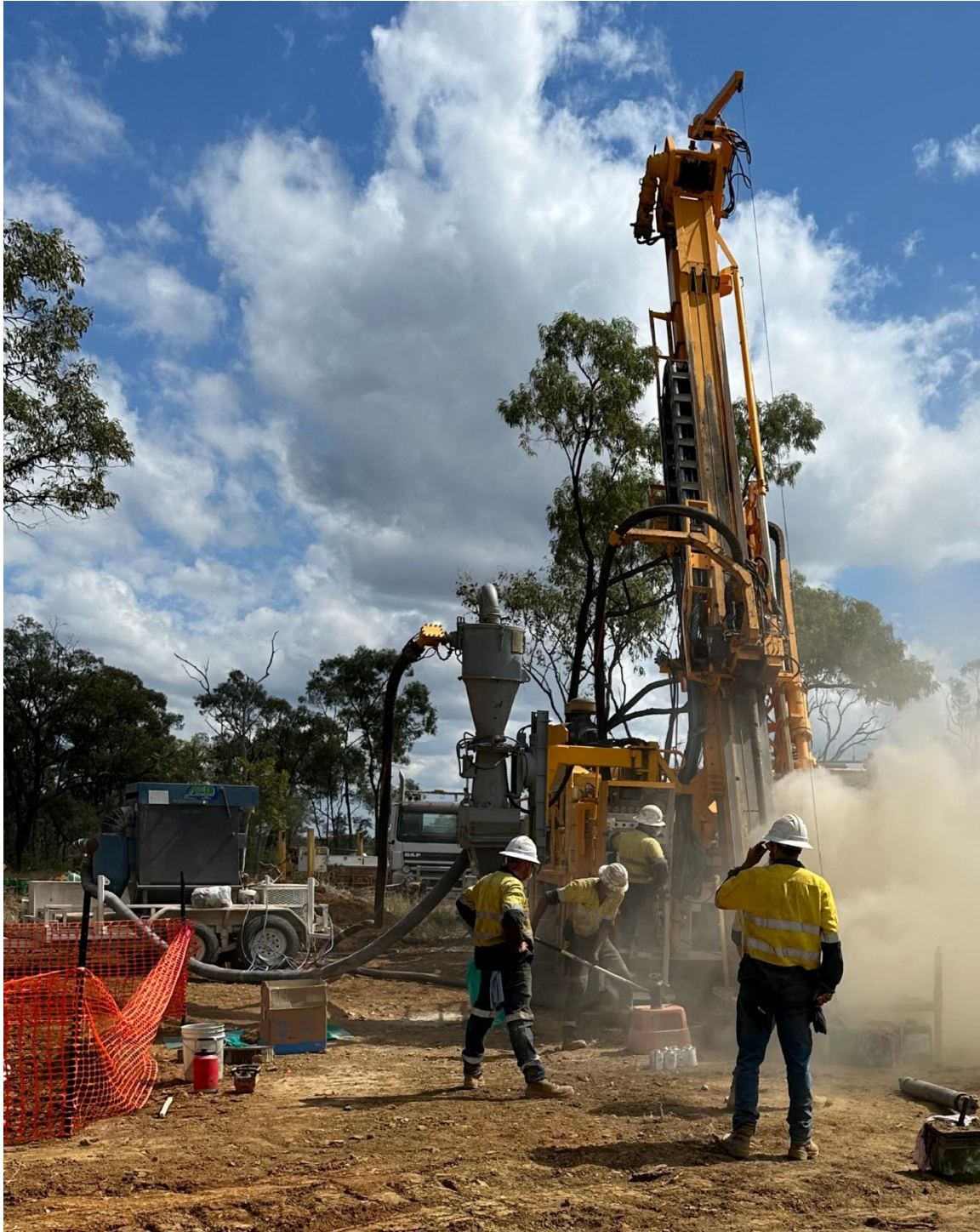
Figure 1 – Drill rig set up and commencing RC collar for drill-hole 25GRV01
