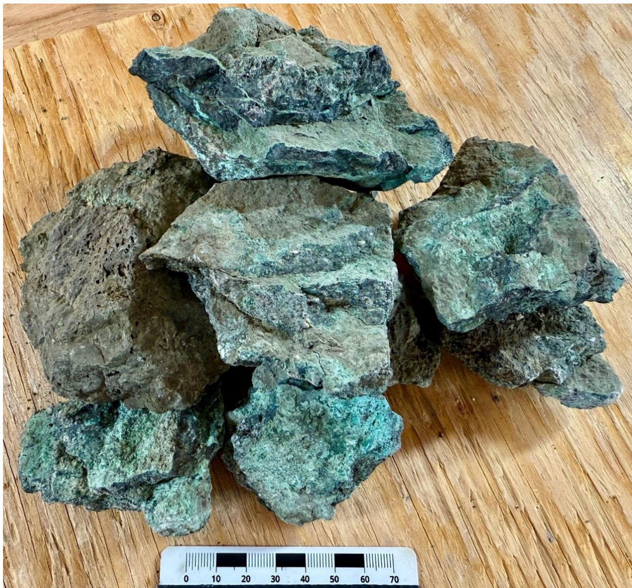
Figure 4 – Photograph of mineralisation observed at observation point id X961216. Amygdaloidal basalt flow top with vesicles filled by chalcocite-malachite and cross cutting chalcocite veinlets. Cautionary Statement: The Company cautions that, with respect to any visual mineralisation indicators, visual observations and estimates of mineral abundance and uncertain in nature and should not be taken as a substitute or proxy for appropriate laboratory analysis. Visual estimates also potentially provide no information regarding impurities or deleterious physical properties relevant to valuations. Assay results from the drilling and sampling programmes will be required to understand the grade and extent of mineralisation. Initial assay results are expected in the September quarter.
