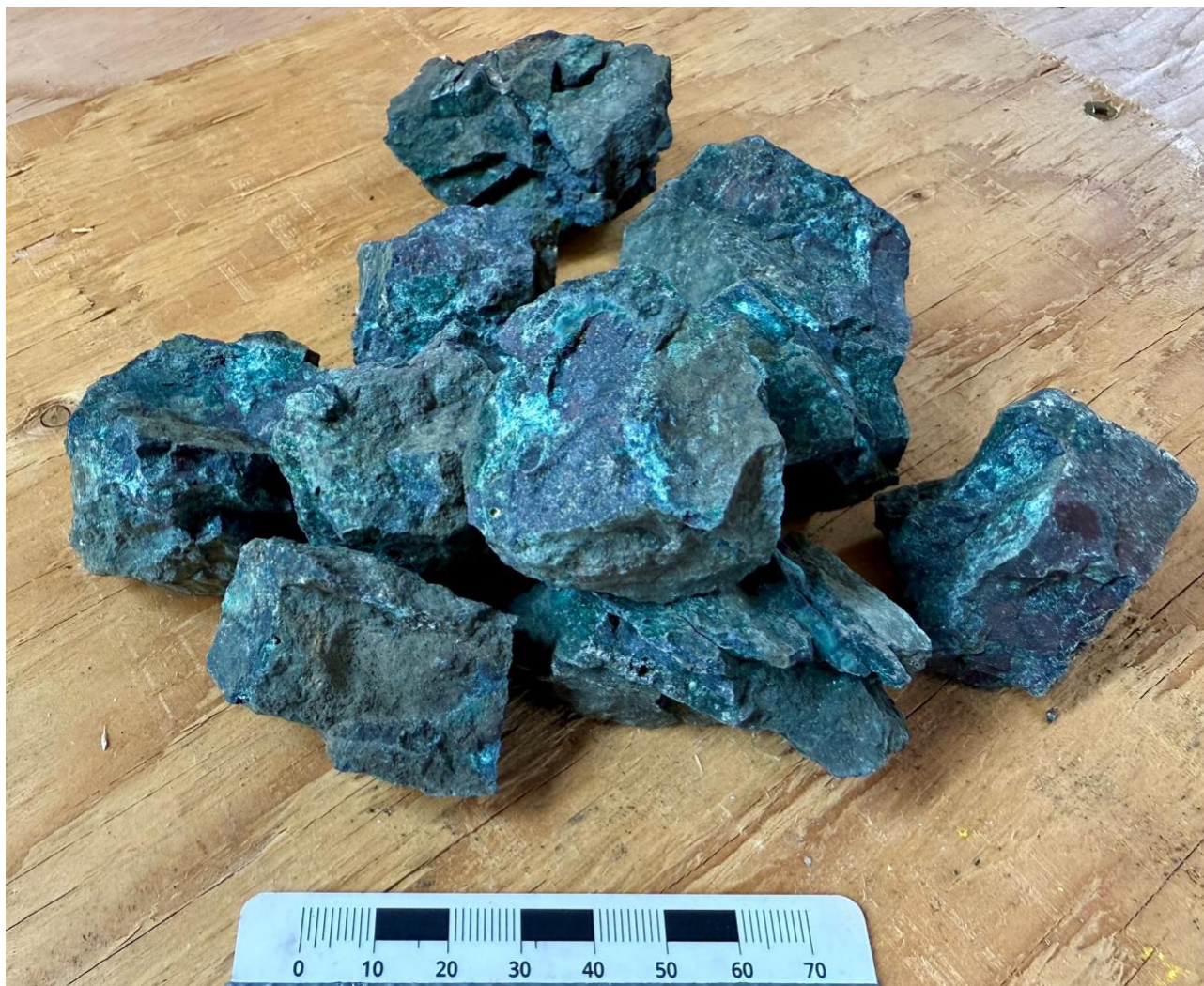
Figure 5 - Photograph of mineralisation observed at observation point id X961205. Massive basalt with chalcocite veinlets and disseminated chalcocite, moderately hematite altered. Cautionary Statement: The Company cautions that, with respect to any visual mineralisation indicators, visual observations and estimates of mineral abundance and uncertain in nature and should not be taken as a substitute or proxy for appropriate laboratory analysis. Visual estimates also potentially provide no information regarding impurities or deleterious physical properties relevant to valuations. Assay results from the drilling and sampling programmes will be required to understand the grade and extent of mineralisation. Initial assay results are expected in the September quarter.
