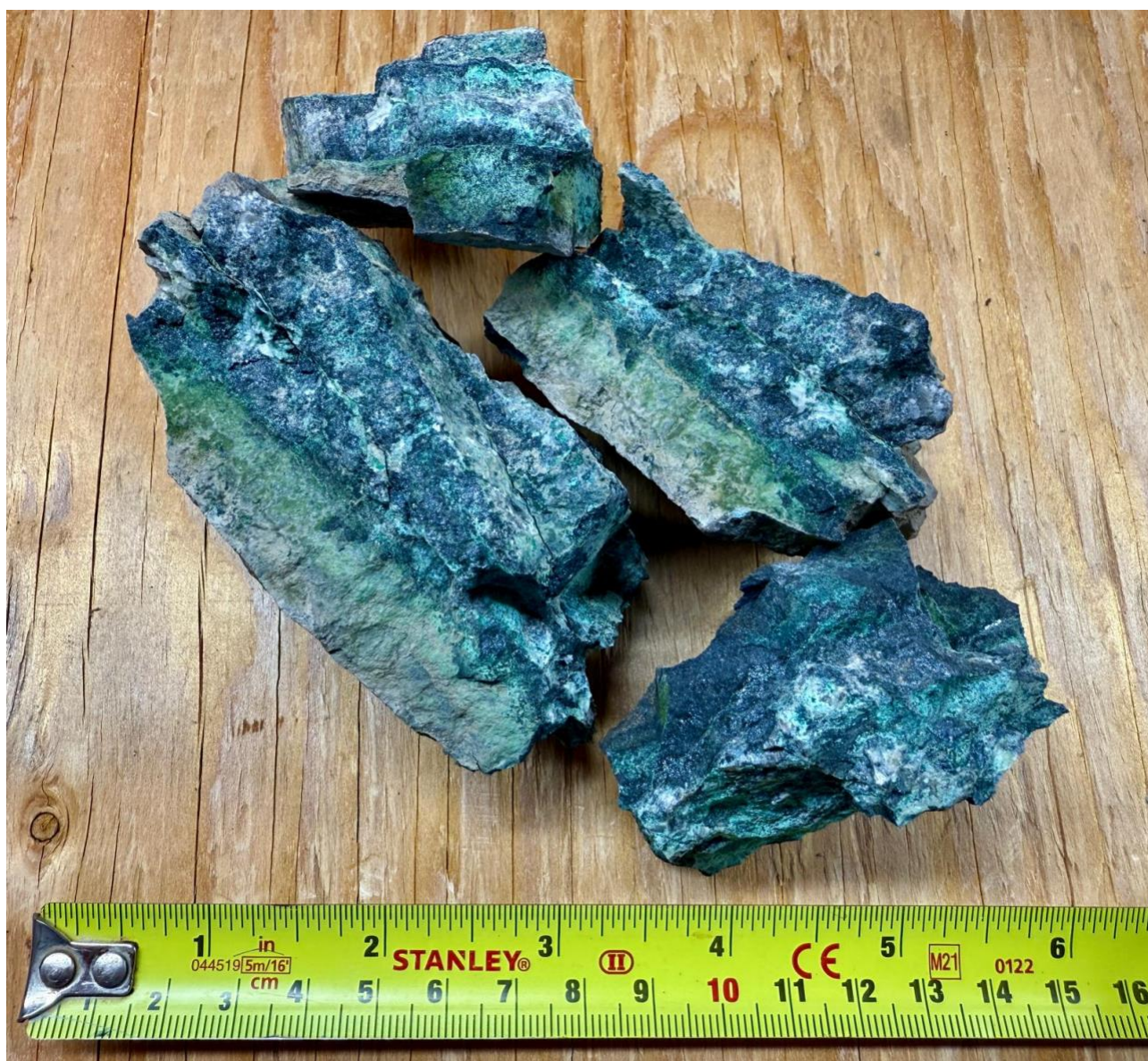
Figure 5 - Photograph of chalcocite (15%) and malachite (3%) within a veined and brecciated basalt located at 521535, 7473411 NAD83 UTM Zone 11N. Mineralisation has similarities with Danvers, over 4km to the NE along a major structure. Cautionary Statement: The Company cautions that, with respect to any visual mineralisation indicators, visual observations and estimates of mineral abundance and uncertain in nature and should not be taken as a substitute or proxy for appropriate laboratory analysis. Visual estimates also potentially provide no information regarding impurities or deleterious physical properties relevant to valuations. Assay results from the drilling and sampling programmes will be required to understand the grade and extent of mineralisation. Initial assay results are expected in the September quarter.
