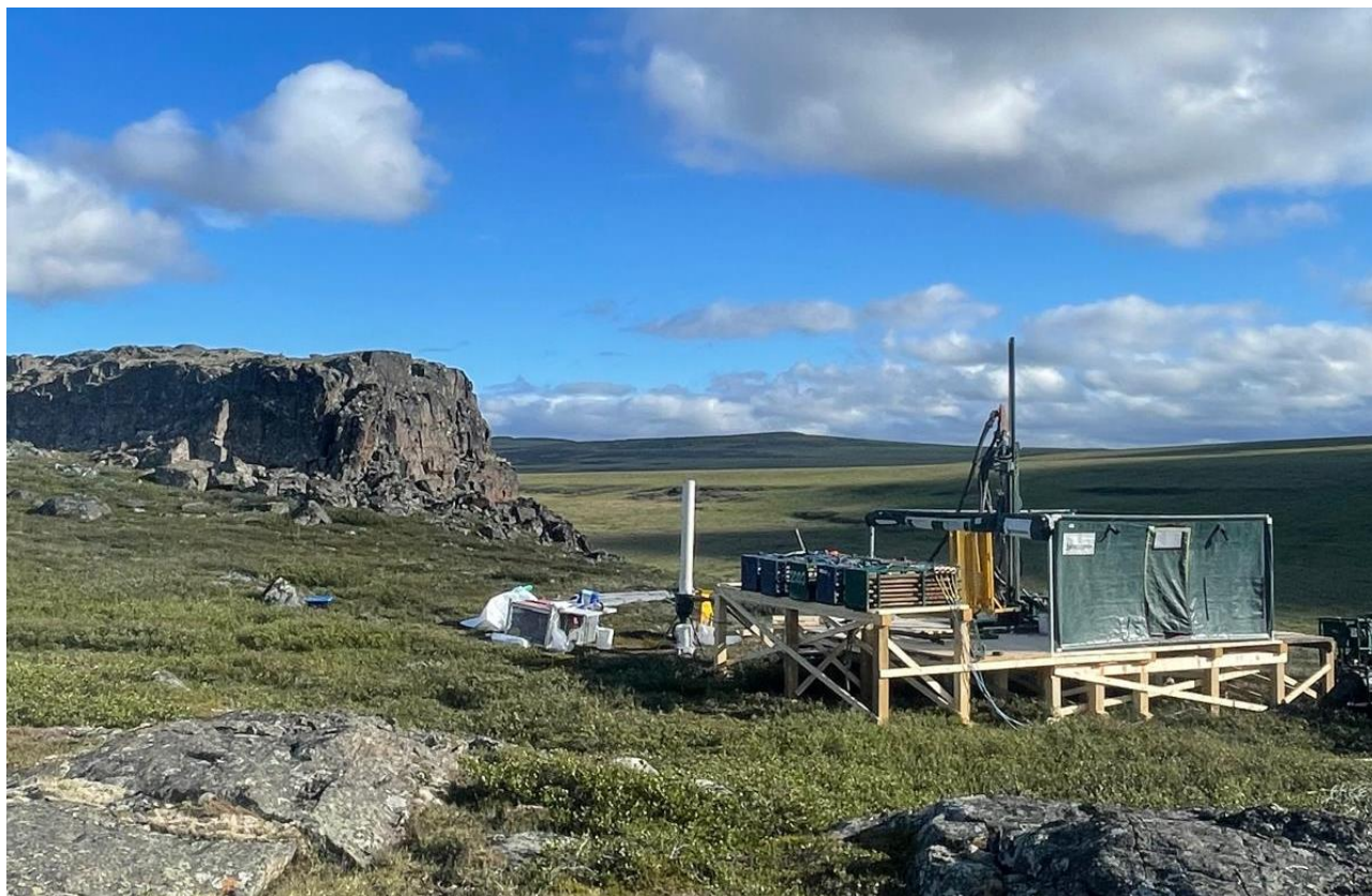
Figure 2 - Reverse circulation drilling underway at the Rae Project site.
