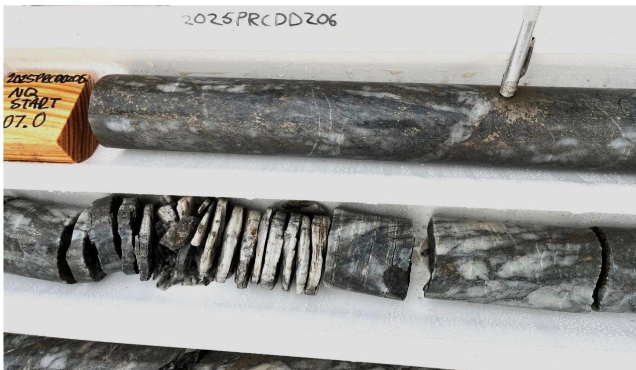
Figure 4 Continuation of the mineralisation of hole 25PRC206 ending in 23.5 g/t at final depth. Core shows quartz-carbonate veining with possible chlorite-amphibole alteration and disseminated to semi-massive sulphides mineralisation with pyrrhotite (ideal for DHEM), chalcopyrite and arsenopyrite characteristic of shear-hosted orogenic gold systems.
