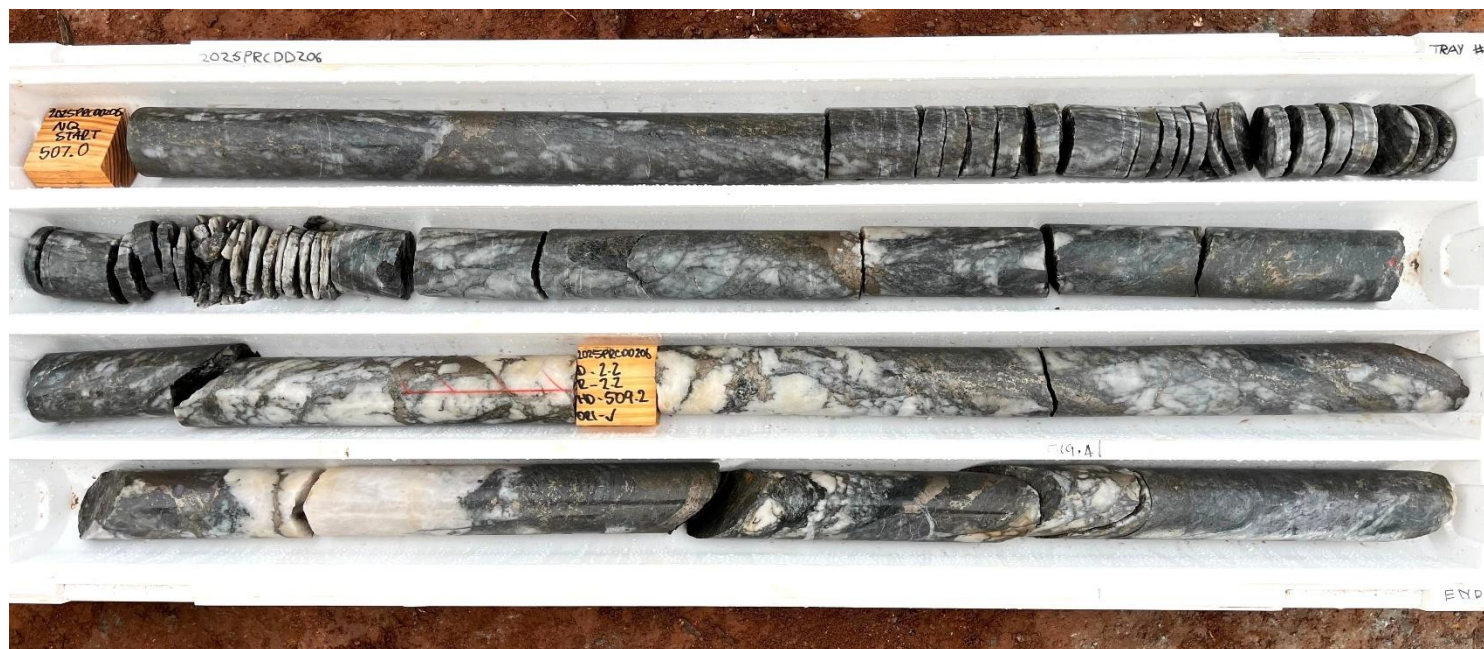
Figure 1 Core tray from hole 25PRCDD206, covering the interval from 507m to 510.9m. Intense, pervasive quartz-carbonate veins, with boudinage, folding, and curved veins, indicating ductile deformation and multiple fluid pulses with sulphides (pyrrhotite, arsenopyrite).
