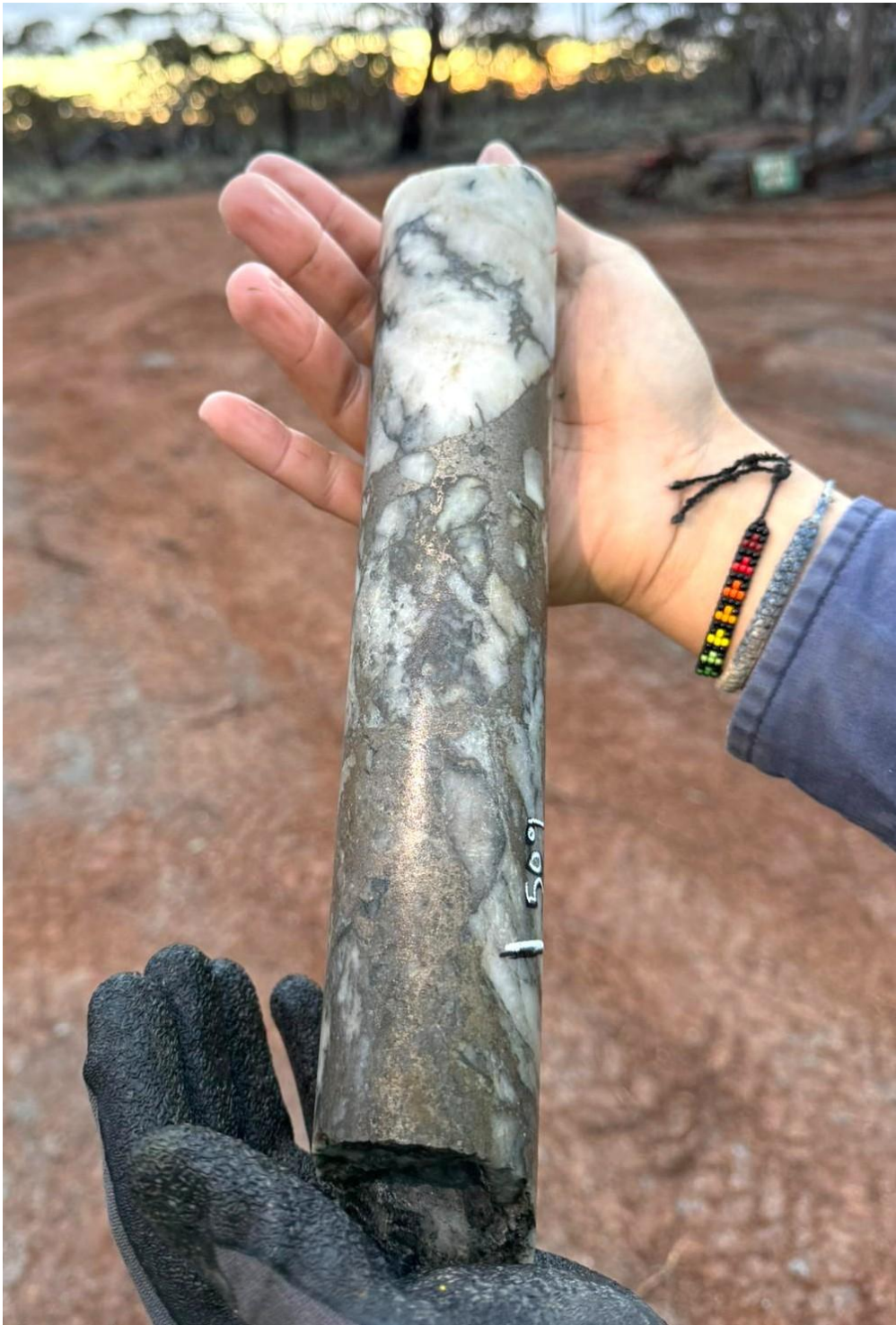
Figure 2 Drill core at 508.80m to 509.2m displaying semi-massive sulphides as pyrrhotite chalcopyrite arsenopyrite breccia with quartz carbonate veining and chlorite alteration. This type of veining and alteration is often associated with orogenic gold systems, especially near structural feeders.
