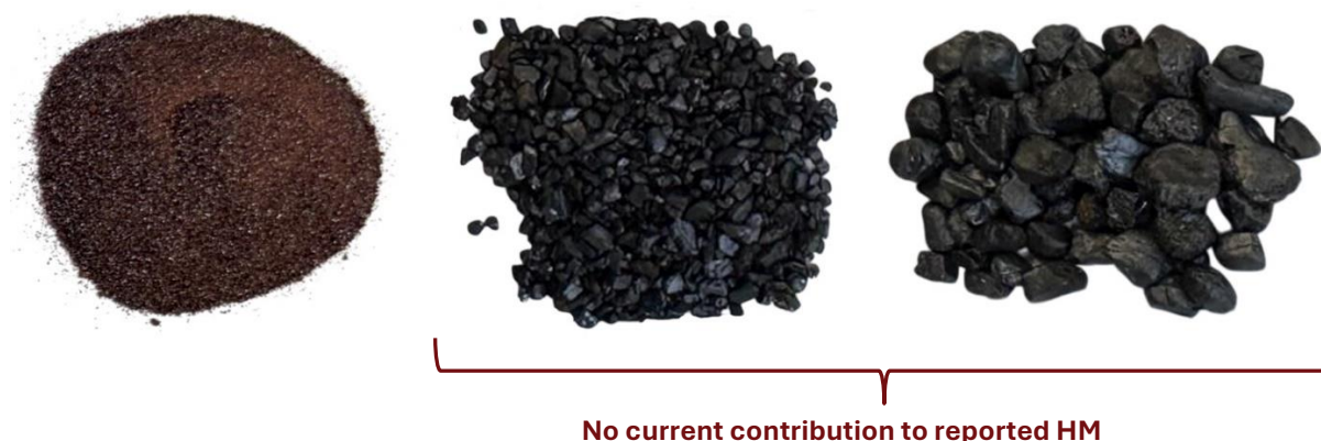
Figure 5: Representation of mineral sand particles versus oversize particles Images from sand and oversized particles are not from Minta area – only shown to demonstrate difference in particle size.
