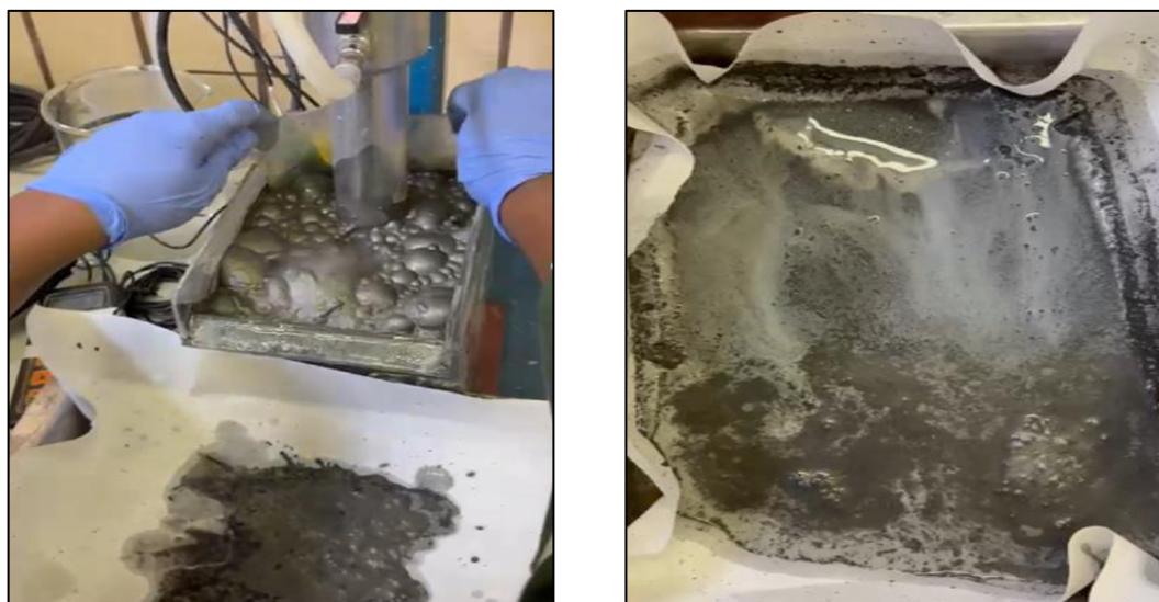
Figure 3: Copper Flotation Test (left) and Copper Rougher Concentrate (right)
