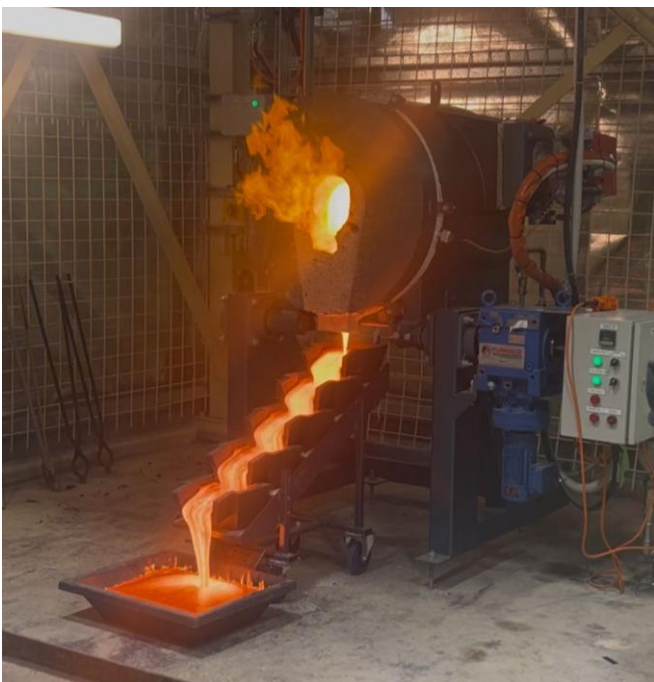
Figure 1: Gold pour via TA100 LPG furnace (30 July 2025)
