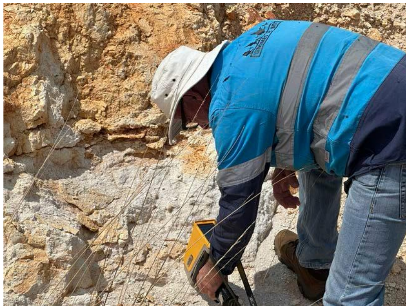
Figure 12. REE Target - pXRF sampling of white weathered kaolinitic fine-grained sediments adjacent to the prominent scarp as shown in Figure 12
