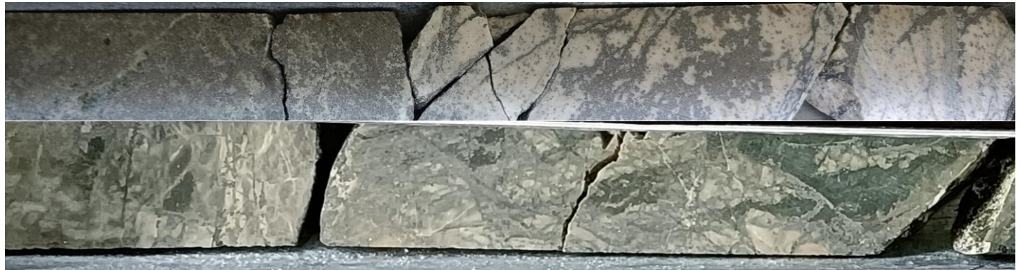
Figure 14 | Mineralised veins in Okvau diamond core. Hydrothermal Quartz Breccia with Arsenopyrite sulphides. Top Photo: RCDD25OKV765- 1m @ 78.30g/t Au from 158m. Bottom Photo: RCDD25OKV712- 1m @ 31.00g/t Au from 212m
