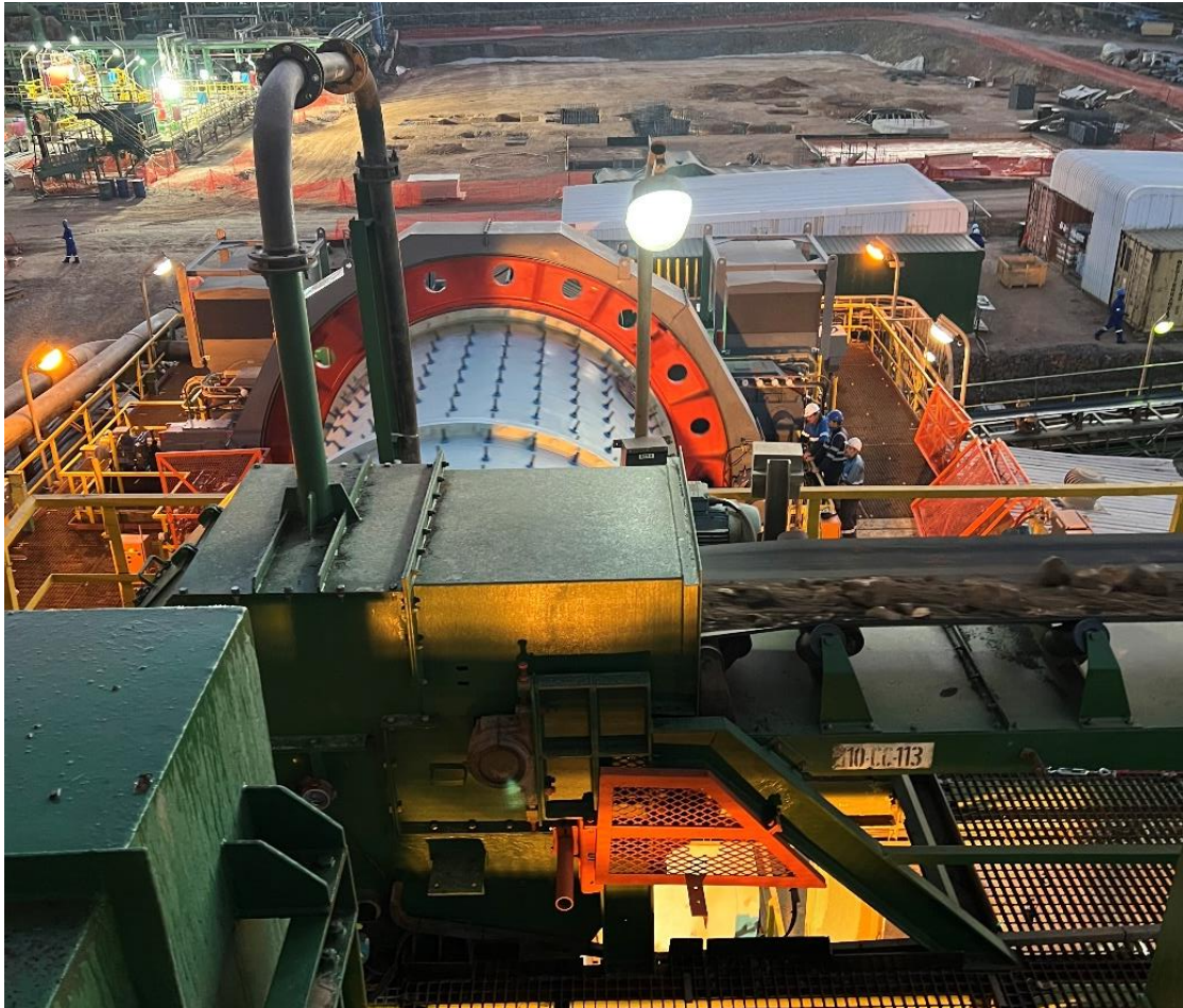
Figure 2: Mineralised waste being fed into the SAG mill
