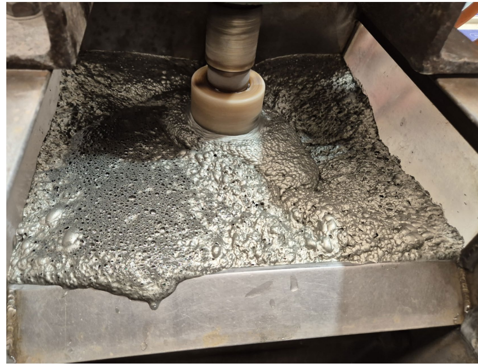
Cleaner flotation – increases gold grade and reduces concentrate mass
