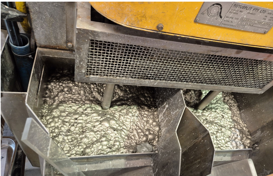
Rougher flotation – recovers as much sulphide as possible to concentrate
