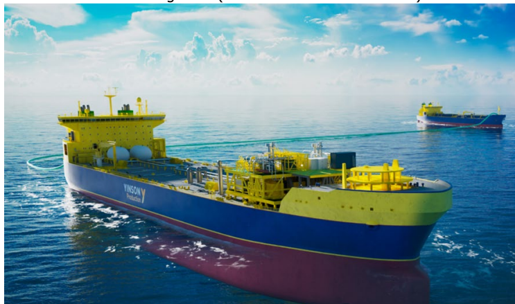
Illustration of a FSIU in the foreground, receiving cargo from a LCO2 carrier in the background (Source: Yinson Production AS)
