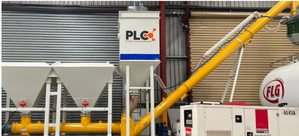
Above: Debagging unit commissioned which provides dust free decanting of quicklime to tankers
