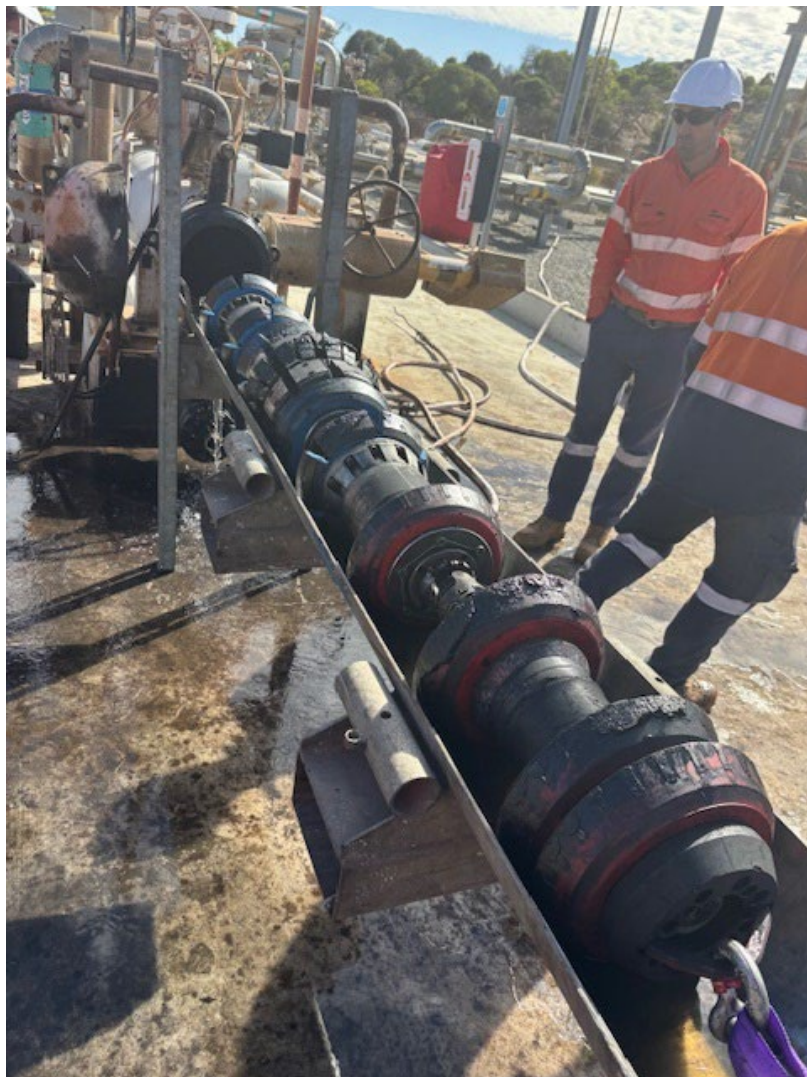
Photo 3: Photo of Intelligent PIG that was run inside the Cliff Head Oil Production and Water Injection Pipelines
