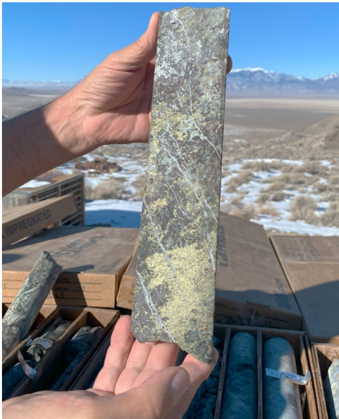
Figure 15: Drill core from WD22-01C from between 421.21-425.33m downhole (3.4% Cu, 91g/t Ag, 0.74g/t Au, 17g/t In, 0.05% Mo - See ASX announcement dated 19 September: Assays Confirm Growth Potential at West Desert). This intersection is located outside of the current West Desert MRE.
