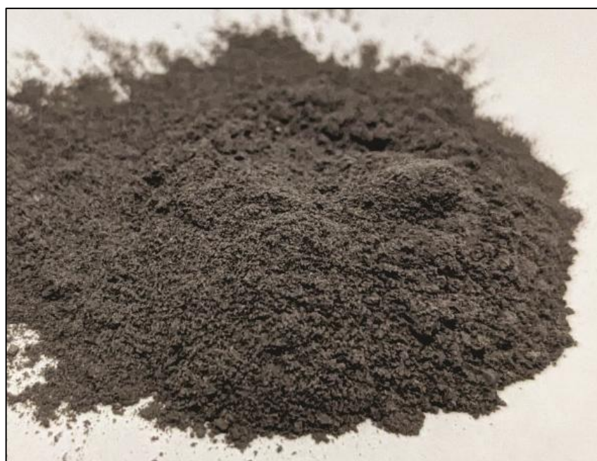
Figure 4: Antimony sulphide (37% Sb) precipitated from leach liquor
