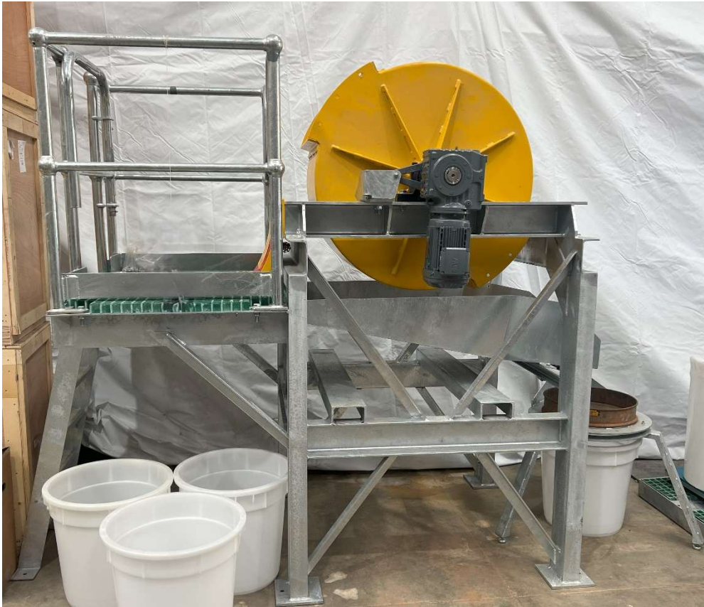
Figure 1 Pilot Plant Scrubber
