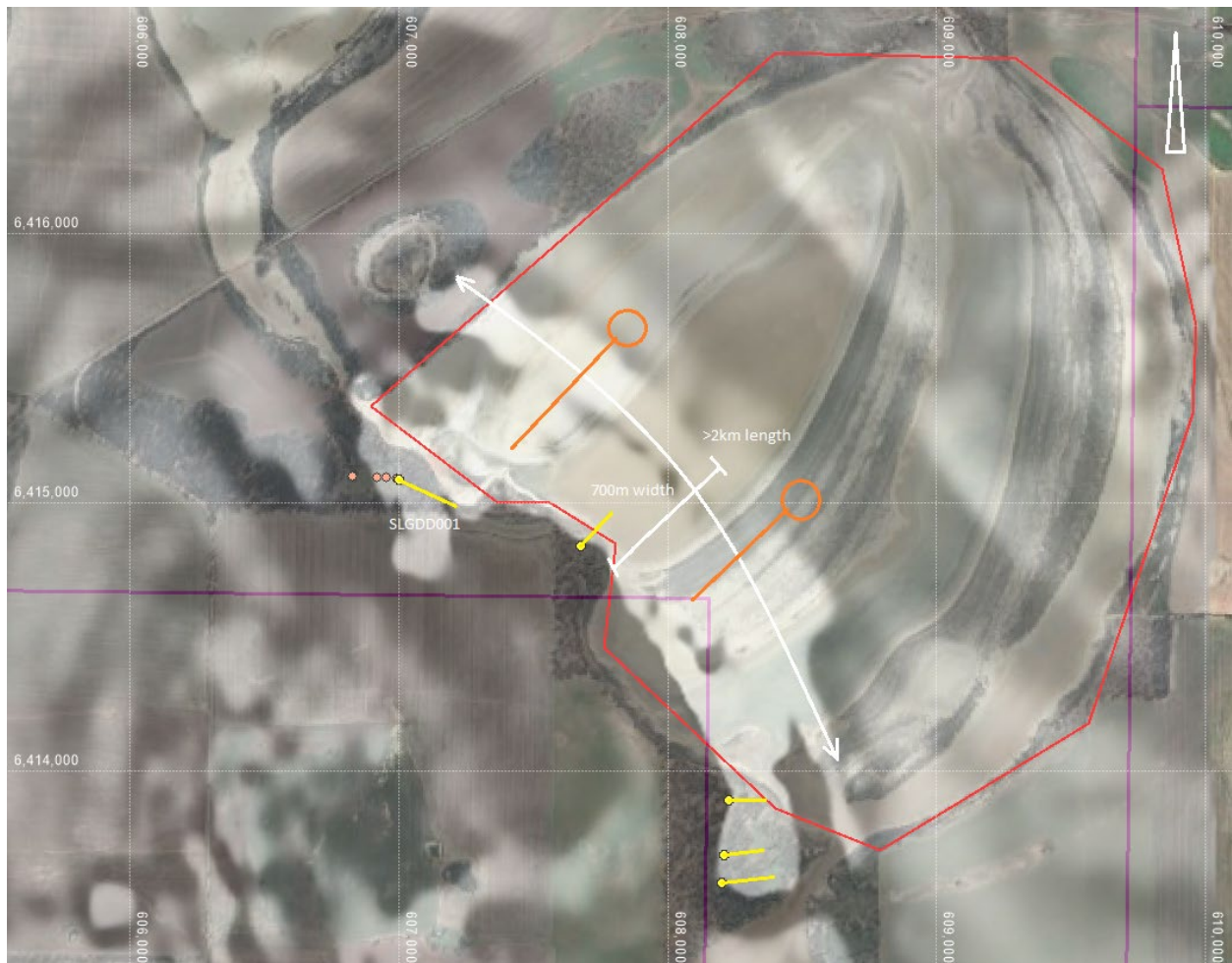
Figure 10: Khal Nickel-Cobalt Project- Plan view of 1VD magnetic signature representing the >2km long, 700m wide ultramafic sequence overlain by aerial photography highlighting the salt lake, with Reserve 18455 (Lot 225568) highlighted in red. Sultan's 2022 aircore collars are marked in orange, and previous diamond drilling traces in yellow, with recent SLGDD001 named. Orange circles and traces indicate possible drilling collar positions to test the layered intrusion from the salt lake surface. An all weather collar position from the SW is also being considered.
