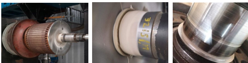
Image 3, left to right: train components on the TKF 9000; motor shaft 'as sprayed'; surfaces machined to final tolerance.
