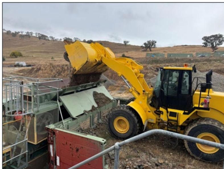
Figure 1: Loader tipping remnant high-grade ore to crushing circuit (GDM ASX Announcement 2 June 2025)
