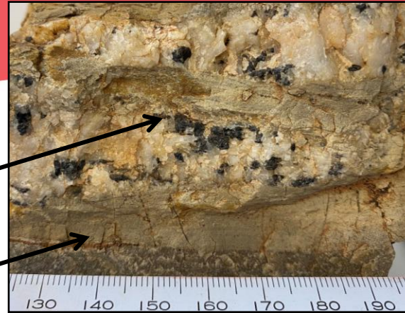
Cassiterite from Tallebung – Scale in mm
