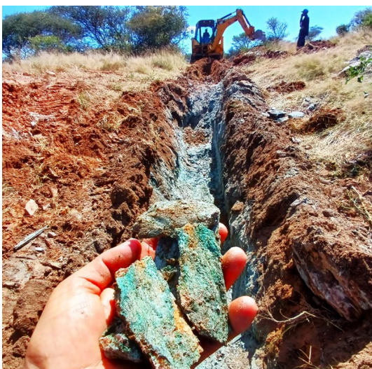
Photo 1: Copper oxide mineralisation in schist – DET003 2-5m
