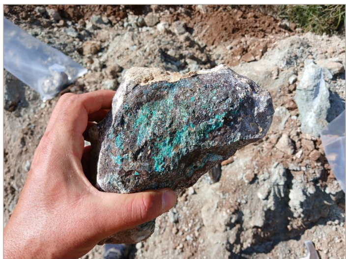
Photo 2: Copper oxides within ferruginous-calcite – DET003 61-62m
