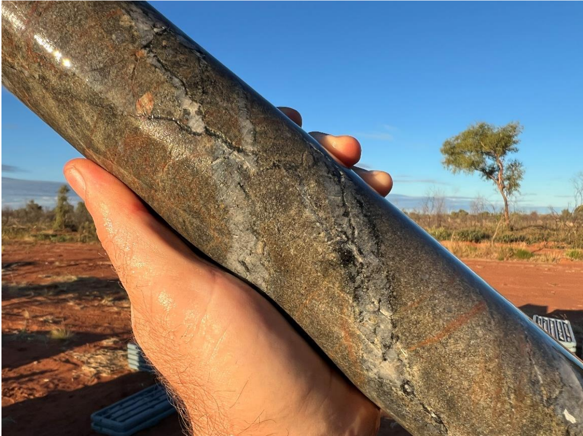
Figure 2. Example of sub-vertical sheeted quartz veins, with typical orogenic style alteration in a diamond drill core sample from 25XCDD001 (twin of 24XCRC097) at 118m down-hole.
