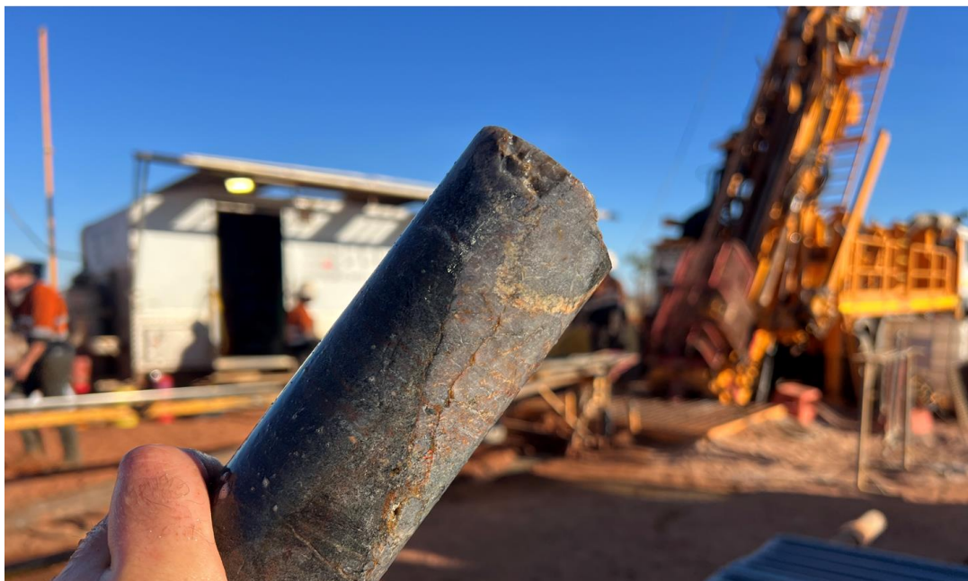
Figure 1. DDH1's rig 25 drilling hole 25XCDD001 at the Martin Prospect, twinning previous RC hole 24XCRC097 (10m at 12.66g/t Au and 10m at 7.34g/t Au), with core in the foreground showing an example of the interpreted sub-vertical high-grade gold bearing stacked quartz vein – assaying and petrographical analysis is planned post structural logging.
