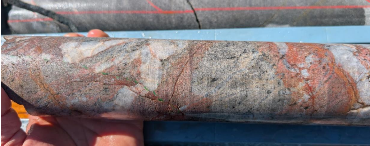
Figure 3. Example of mineralisation typical of the interpreted broad lower-grade gold in 25XCDD002 (twin of NEWXCRC015) at 91m down-hole, where NEWXCRC015 returned 38m @ 0.22g/t Au from 82m.
