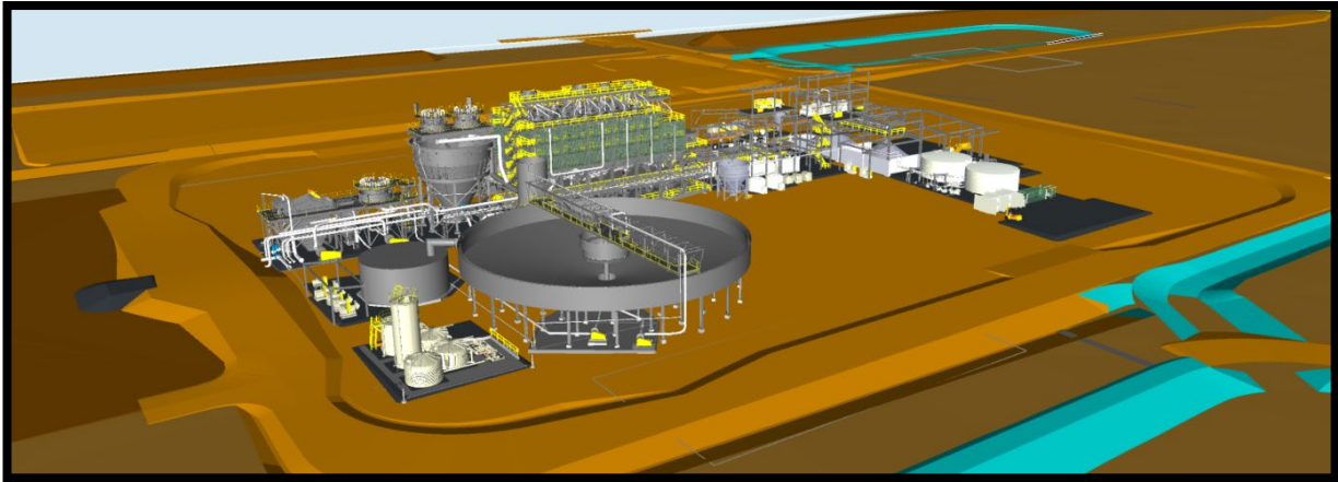
Figure 18 – Thickener and process water ponds
